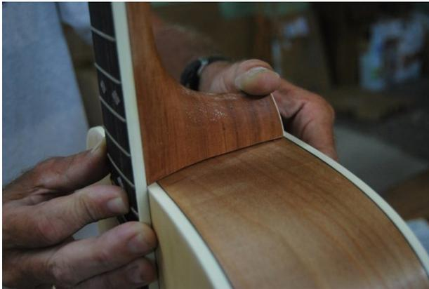
Apply plenty of glue in the neck joint and to the neck, where it will be in the joint. Then, place the neck in the joint and clamp it tightly. If glue doesn't squeeze out all around the joint, you haven't applied enough glue. Once you have the clamp(s) set, use a soft cloth wet with warm water to remove any excess glue. The glue sets up fairly quickly, but you have a few moments to check the neck to be sure it's where you want it to be.
