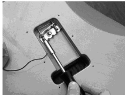
Next solder the tremolo ground wire onto the spring claw.
