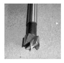
A forstner bit is the ideal bit. It has a small pilot point so it's easy to center up, but it drills a clean, flat-bottomed hole. So, now you know how to do it; drill the two stud anchor holes, about 1 inch deep, centered on the marks you made earlier.
