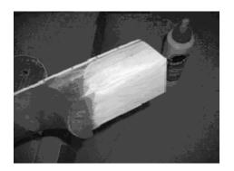
Then, place the neck in the joint and clamp it tightly. If glue doesn't squeeze out all around the joint, you haven't applied enough glue. Once you have the
