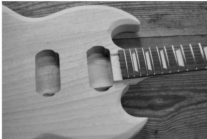
Test fit the neck and be sure that your clamp(s) will hold the neck securely. If you use some cardboard or something to pad the clamp, be sure no glue gets on it; it will be almost impossible to remove without damaging the guitar. Apply plenty of glue in the neck joint and to the neck, where it will be in the joint.
