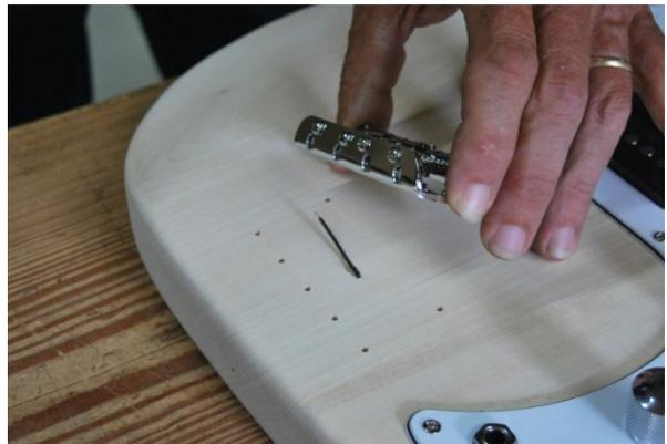
Secure the bridge to the body with the screws provided.
